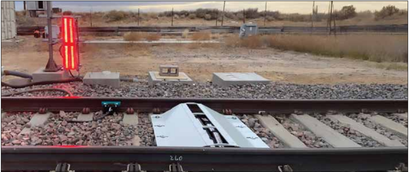
KLD's newest products, UnderScan and SillScan, produce high resolution images of the underfloor and side views of rolling stock.
