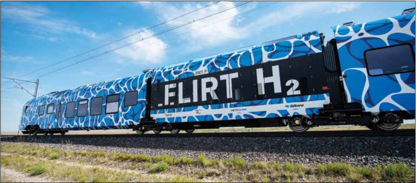
Stadler's FLIRT H2 hydrogen fuel cell electric train on its record-breaking run at the FRA's Transportation Technology Center in Pueblo, Colorado.
