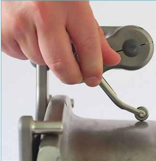
KLD Labs offers both automated and portable measurement tools for assessing wheel profiles and wheel wear conditions, as well as tools for condition-based maintenance planning and execution. While WheelScan™ is the automated solution, MiniProf BT Wheel is the portable version designed for quick and accurate wheel profile measurements.
