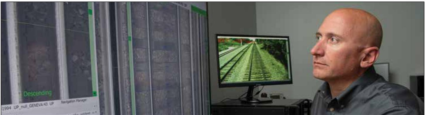
ENSCO's VTW software allows high-resolution track images to be inspected in the office. A key feature is the ability to view synchronized images from multiple inspection cameras, along with milepost and GPS data. VTW provides tools for marking defects and identifying track assets, which are then automatically tagged with milepost numbers and GPS coordinates. Identified defects and assets can be exported to CSV reports.
