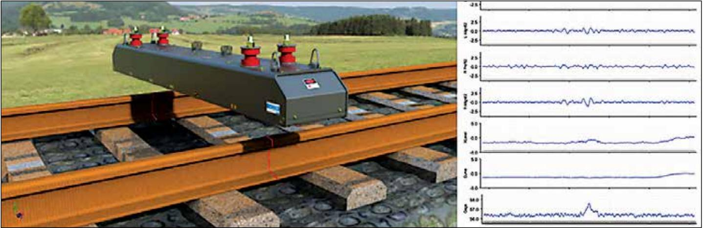
Track geometry measurement is a crucial method in the rail industry for assessing track safety and planning maintenance. Regular measurement and analysis of track geometry are proven to prevent track-related derailments, which can cause catastrophic damage. ENSCO's TGMS leads the industry in reliability and measurement reproducibility.
