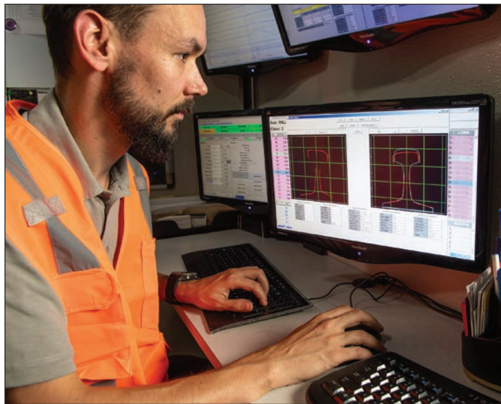
ENSCO staff can operate and maintain your track inspection technology on your behalf.
