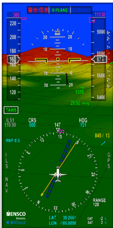
Portrait Synthetic Vision version of Primary Flight Display with Terrain Awareness Warning enabled, created with IData and IDataMap.
