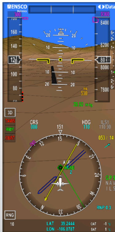
Portrait Synthetic Vision version of Primary Flight Display, created with IData and IDataMap.
