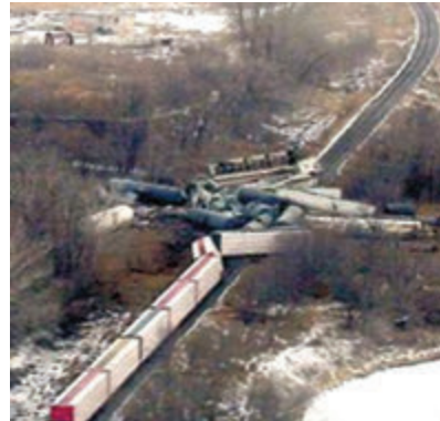
Aerial photo of the 2002 Minot train derailment caused by a broken joint bar
