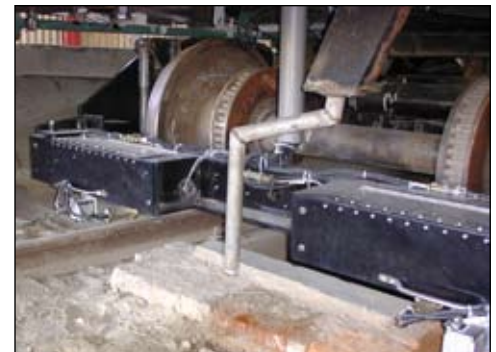
Gage and corrugation sensors of the two sets is visible on the far end of the sensor beam (black finish). System installed on Indian Railway High-speed Track Recording Car
