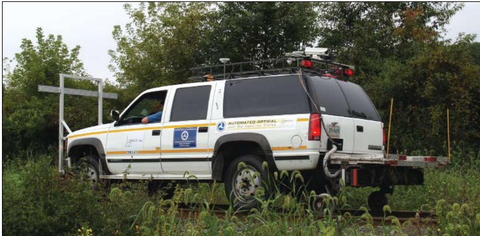
The Track Asset Mapping System utilized on the Hy-Railer.
