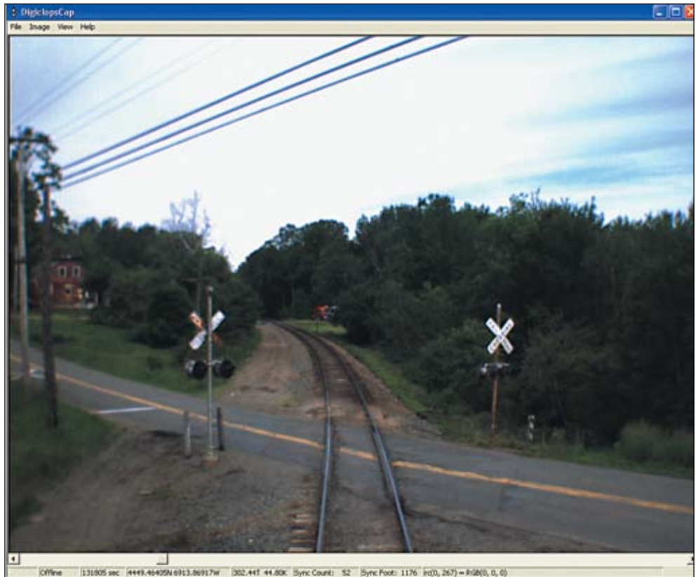
The Track Asset Mapping System provides georeferenced images and locations of your Track and Wayside assets.
