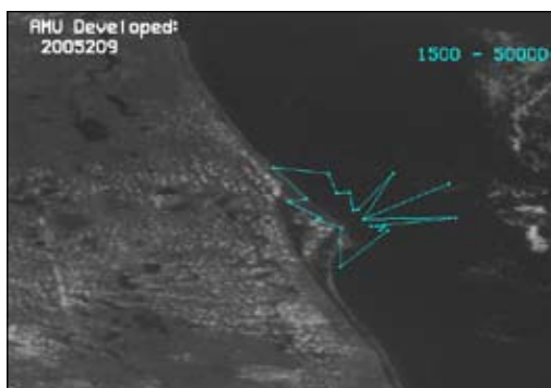
Geographical pattern of camera zones susceptible to cloud obscuration for the network of long-range cameras used during Shuttle launches from Kennedy Space Center. The zones are valid for high clouds with bases at 18000 ft and tops at 30000 ft. The satellite image shows high clouds in the area.
