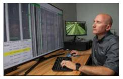
Software enables high-resolution, synchronized track images to be inspected in the office
