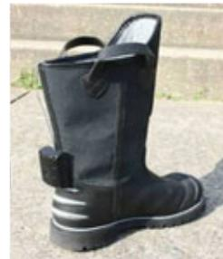
**Figure 13: IMU mounted on heel of firefighter's boot.**
