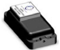
The core processing includes an extended Kalman filter (EKF) to integrate zero-velocity and heading observations with the position, velocity and attitude based on the integrated inertial navigation equations for each IMU measurement. The EKF state vector consists of the following 15 states:
