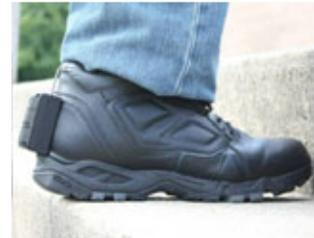
Figure 4: MEMSense nIMU mounted on operator's boot.
